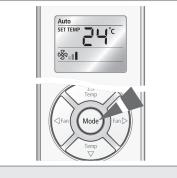
3 To adjust the temperature, press Temp v button to set the desired temperature. The temperature can be set between 18°C(65°F) and 30°C(86°F).
